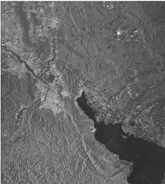
Figure 3 PALSAR Multi-look Intensity Image over Kyoto acquired on 21-Mar-2006 by ALOS in Fine-Beam HH pol. mode.
