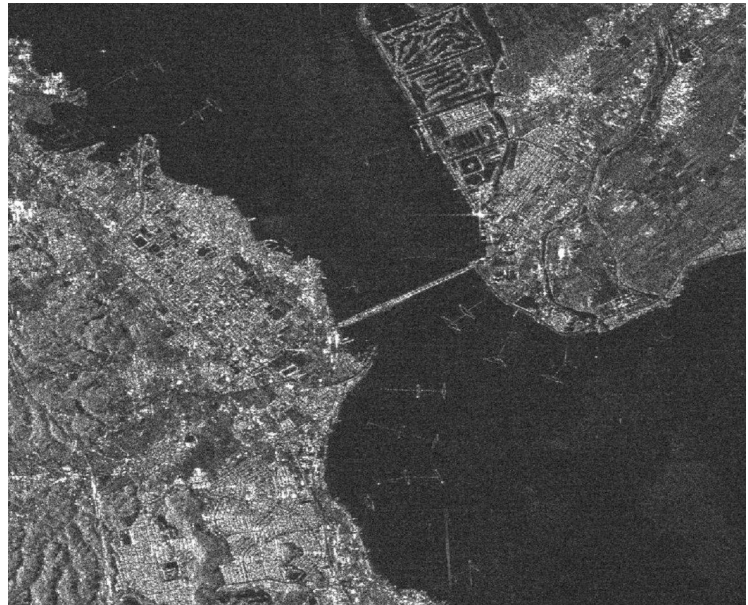
Figure 4 Full range resolution section of the PALSAR Kyoto image acquired on 21-Mar-2006. The slant range sampling corresponds to an approx. ground range sampling of 7.9 m, the azimuth pixel spacing (3-look) is 9.55 m.
